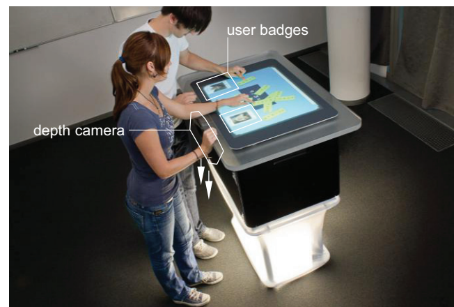
Figure 1: Bootstrapper recognizes users interacting with the table by observing their shoes using depth cameras.
